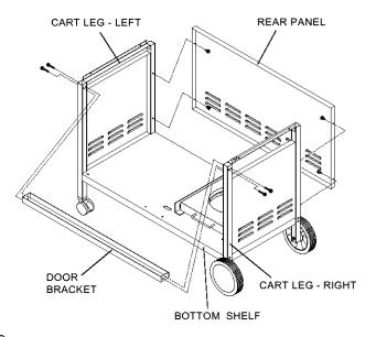
7. Install the Door Bracket to the inside of front Cart Legs. Align the threaded holes on the Door Bracket with the holes on Cart Legs. Tighten securely by using 4 of the 1/4"x2" Pattern Head Screws provided. (See Fig. 3. on page 11) Upper door bolt holes (at ends of bracket) must face outward.
